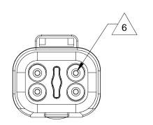
STRAIN RELIEF END CAP -BLACK - ALL — CONNECTORS RECEPTACLE, 4 PIN, AT SERIES, STRAIN RELIEF END CAP
